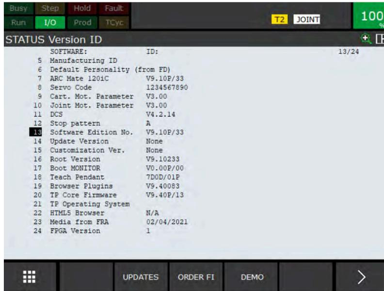
7 Look for the required options. Under "Continue displaying?", press **YES** to see more of the installed options. If any of your controller's required options are missing, contact your FANUC distributor to upgrade.
