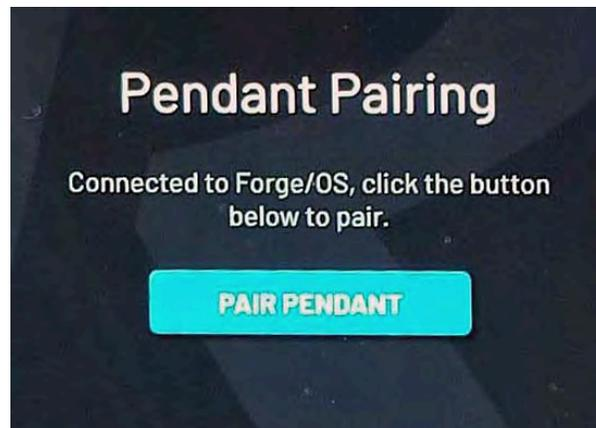
**Note:** If the pendant fails to pair or the **PAIR PENDANT** button is unavailable for longer than two minutes, check the Ethernet connection to the **IPC**. If the pendant still doesn't pair, connect the pendant's Ethernet cable to another LAN port on the **IPC**. The **READY pendant** IP Address is preset to 172.16.255.253. The network interface that the pendant connects to should use IP Address 172.16.255.250 and Subnet mask 255.255.255.0.
