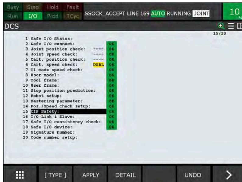
**d** In the CIP Safety menu, set **Enable/bypass** to "ENABLE." Set both the input and output sizes to "2."
